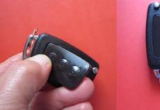
Place a new silicone pad over top part of your remote. Use rolling motion when positioning pad in grooves and press firmly till pad "engages" with hard shell all around edges. DO NOT USE any lubricants or detergents for cleaning grooves as it will affect firm seating of a pad.
