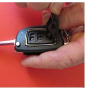
**Do Not open remote.** Gently remove an old rubber pad from your remote using flat screw driver.
